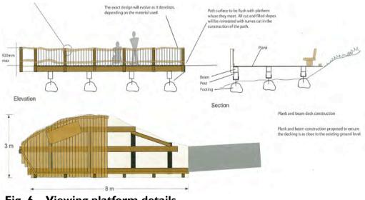
Fig. 6 - Viewing platform details
